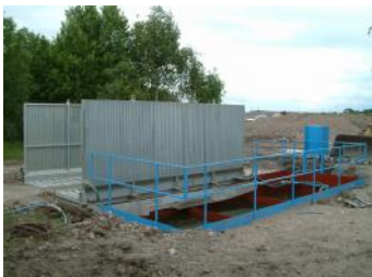
FORCE SIX WASH DECK WITH CONCRETE DECANTATION PIT AND RAMPED LOADER ACCESS FOR SPOIL REMOVAL
