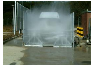
FORCE SIX WASH DECK WITH CONCRETE DECANTATION PIT AND RAMPED LOADER ACCESS FOR SPOIL REMOVAL
